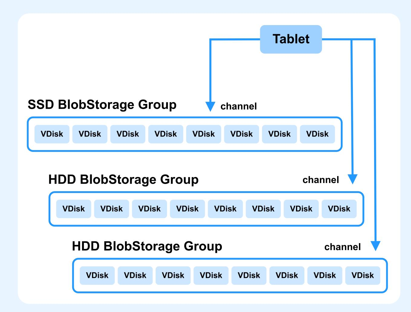
**Tablet** has multiple channels that can be attached to the same or different BlobStorage Groups
