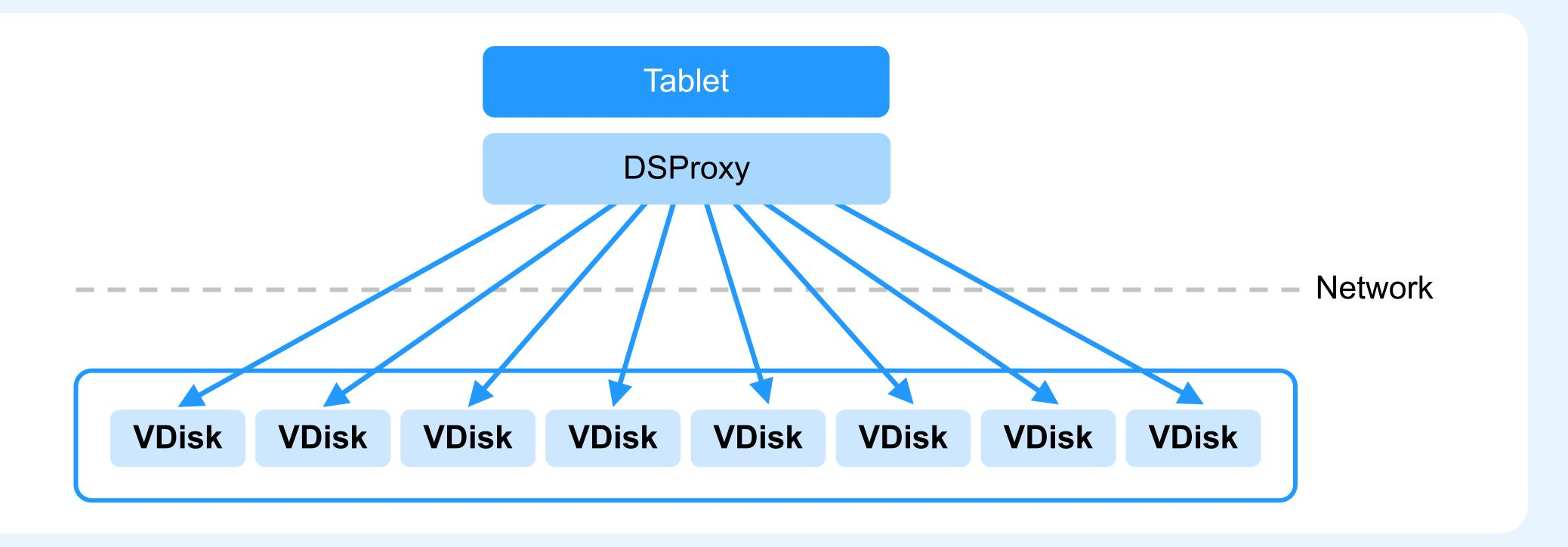
DSProxy communicates with remote VDisks, handles network and disk failures
